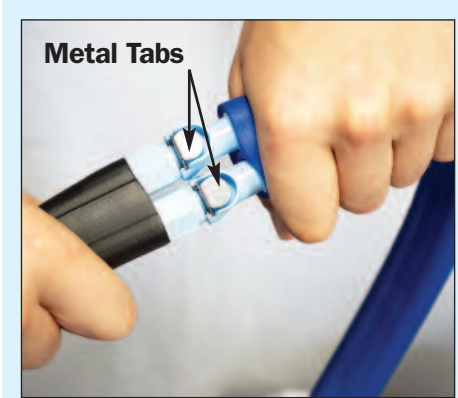
Be sure the metal tabs on the female couplings are pushed down. Then insert the male couplings from the pad hose into the female couplings of the cooling reservoir hose. Insert one at a time. There should be an audible “click” when the couplings are properly seated.
